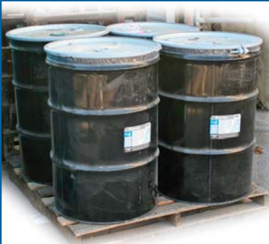
Four 55-gallon drums of epoxy coating — three base and one hardener — wait on a pallet for pickup.
